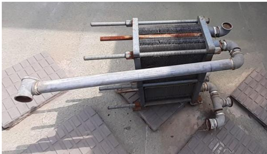
Figure 4-23: Damaged SWH heat exchanger due to scale and fouling formation caused by the hardness of inlet ground source water
