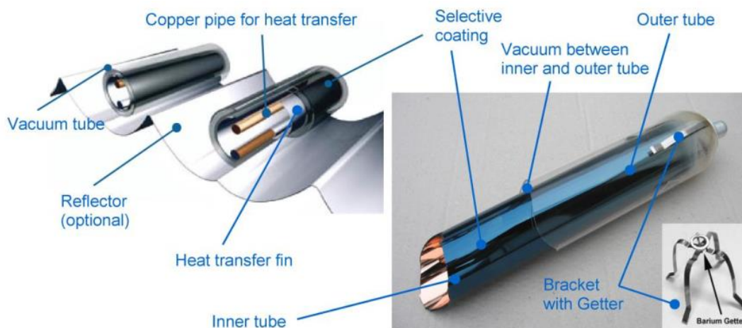
Figure 2-8: Basic elements of a Sydney tube collector (Weiss and Rommel, 2008)
